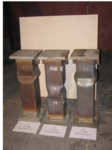
Figure 3. Tests on RHS with slender cross-sections Left: Test specimen in furnace, Right: Test specimens after fire tests (RHS 150x150x3)
