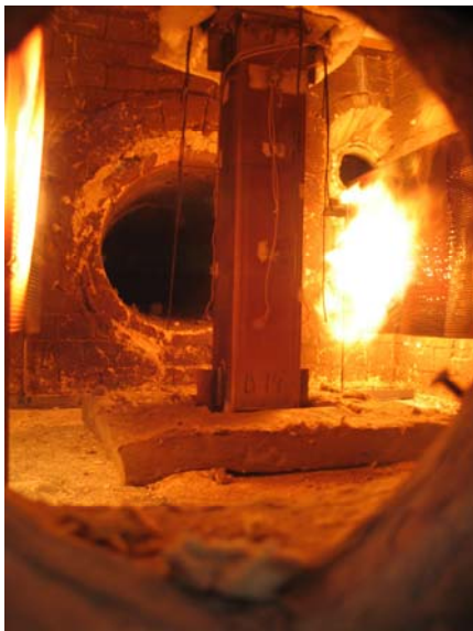
Figure 3. Tests on RHS with slender cross-sections Left: Test specimen in furnace, Right: Test specimens after fire tests (RHS 150x150x3)
